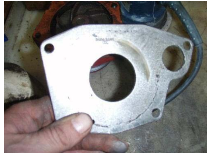
17. Coat the contact surfaces of the water pump assembly with high-temp RTV silicone sealer, and install with new gaskets included with the serpentine pulley kit.
