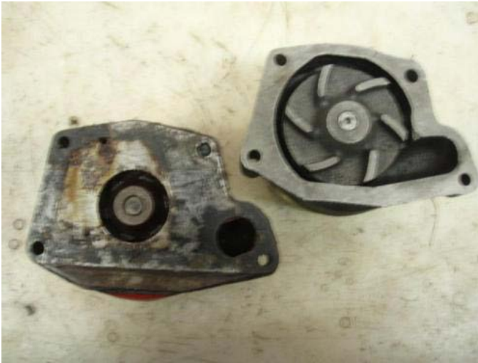
14. Old and new pumps are shown side-by-side. The gasket plate between the old pump and engine block will need to be removed, cleaned, and re-installed with the new pump.
